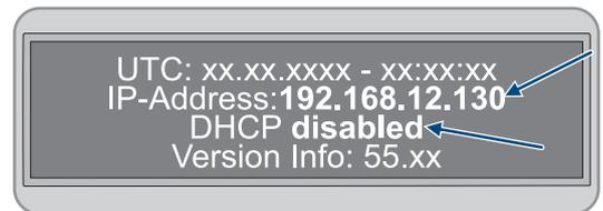
17. If the DHCP protocol is enabled on the battery management system and the IP address is variable, do not make any changes to the configuration of the battery communication during commissioning of the inverter. The default battery communication settings will be automatically used.
