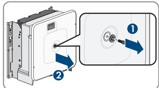
6. Set the cover, screw with seal, washer with seal and enclosure lid aside and store safely.
