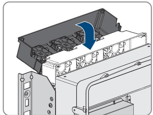
7. Guide the fan bracket on the enclosure vertically downwards into the enclosure brackets provided.
