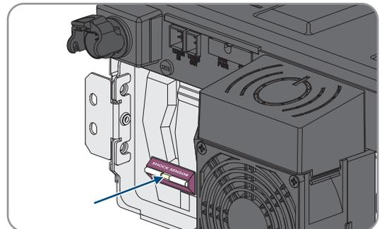
3. If the shock sensor on a battery module has tripped, document the battery module condition using photographs and contact Service. Do not install the affected battery module.
