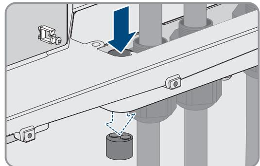
6. For the battery data cable, remove a plug from one of the enclosure openings and for the battery data cable cut an enclosure opening with a utility knife.
