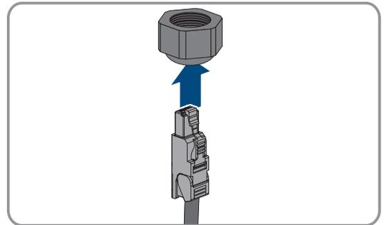
4. Remove the two-hole cable support sleeve from the cable gland.
