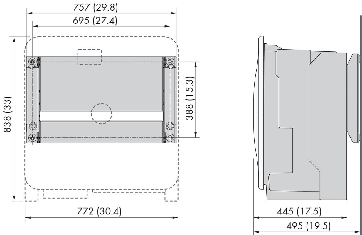
Figure 16: Position of the anchoring points (dimensions in mm (in))
