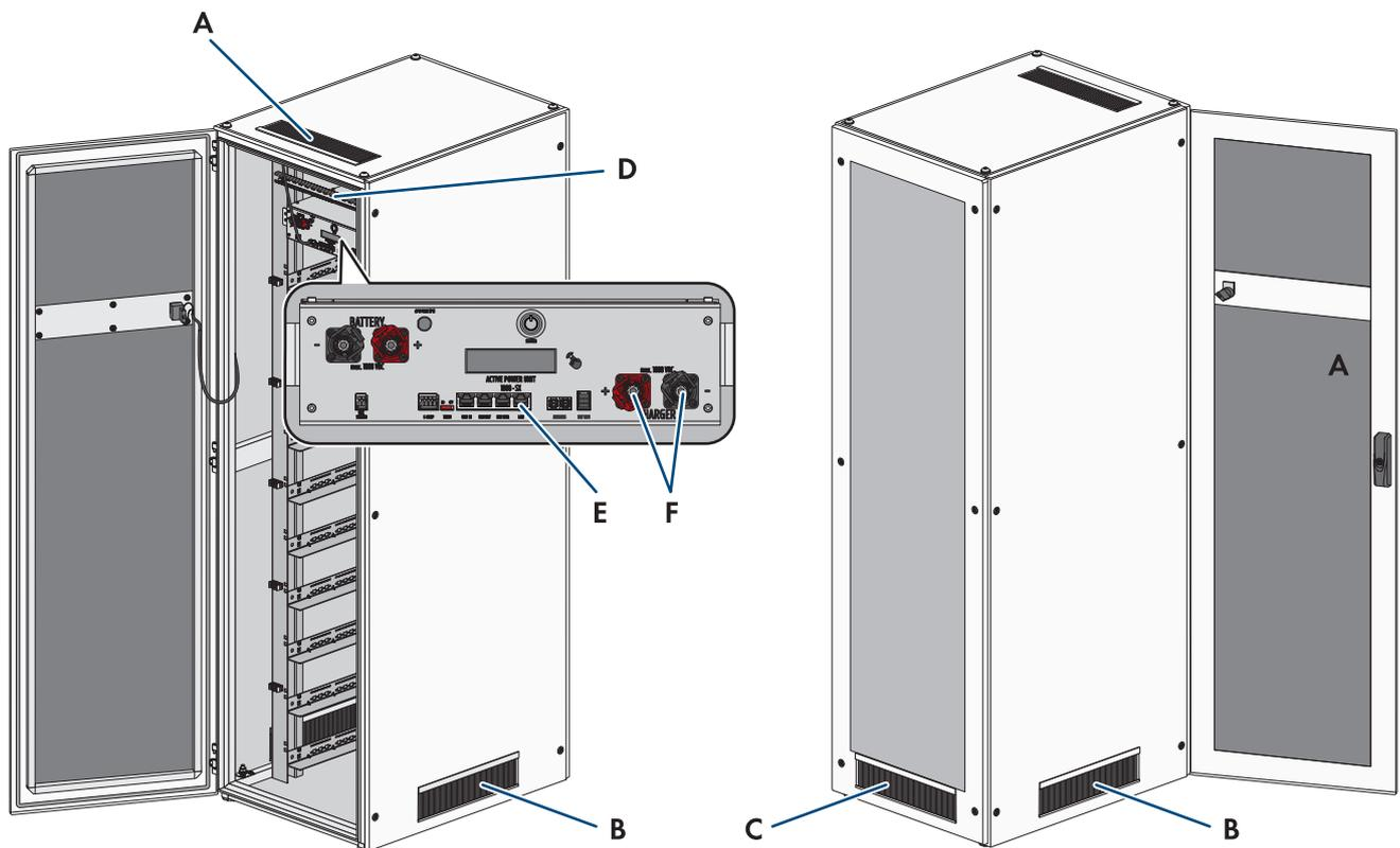
Figure 32: Cable entries in the battery cabinet
