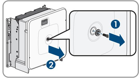
3. Unscrew the swivel nut from the cable gland.
