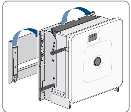
6. Remove all 4 transport handles from the tapped holes. If necessary, insert a screwdriver into the holes on the transport handle and use the screwdriver to remove the transport handle.
