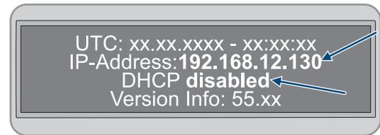
13. If the DHCP protocol is enabled on the battery management system and the IP address is variable, do not make any changes to the configuration of the battery communication during commissioning of the inverter. The default battery communication settings will be automatically used.
