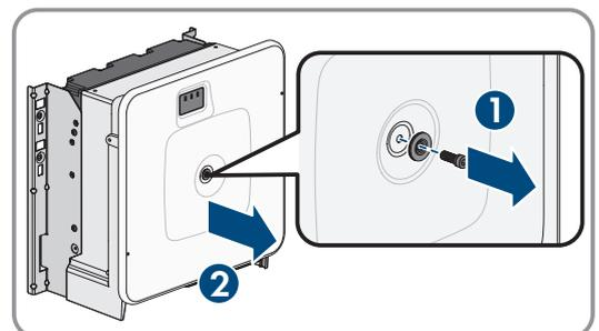
8. Set the screw, cover and cover of the enclosure aside and store safely.
