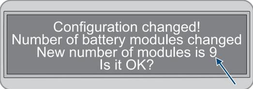
6. If the number of battery modules detected is still incorrect after eliminating any battery communication faults, contact Service.
