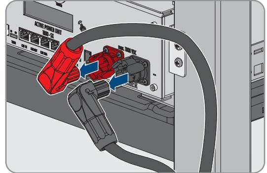
5. Use a suitable measuring device to ensure that no voltage is present at the **CHARGER+** and **CHARGER-** connections.
