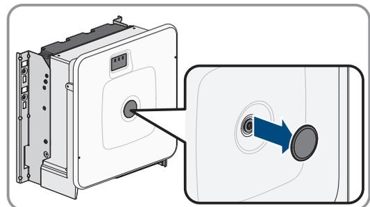
5. Unscrew the screw on the enclosure lid (hex socket, AF8) and remove the enclosure lid.
