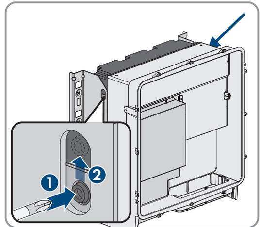
3. Move the fan bracket upwards and fold it backwards. When doing this, note that the fan bracket cannot be removed completely, because the fan cable connects it to the product.
