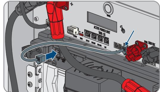
3. Plug the 6-pole connector of a communication cable from the supplied module connector set into the **COMM OUT** socket on the uppermost battery module.
