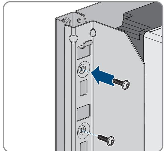
9. Remove all 4 transport handles from the tapped holes. If necessary, insert a screwdriver into the holes on the transport handle and use the screwdriver to remove the transport handle.
