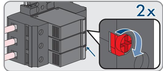
7. Ensure that each surge arrester is securely inserted into its slot.
