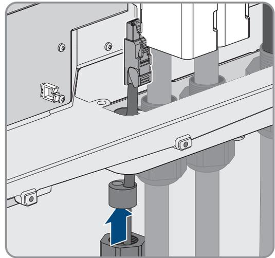
8. When using self-assembly cables, assemble the RJ45 connectors and connect them to the cable (refer to the documentation of the connector).
