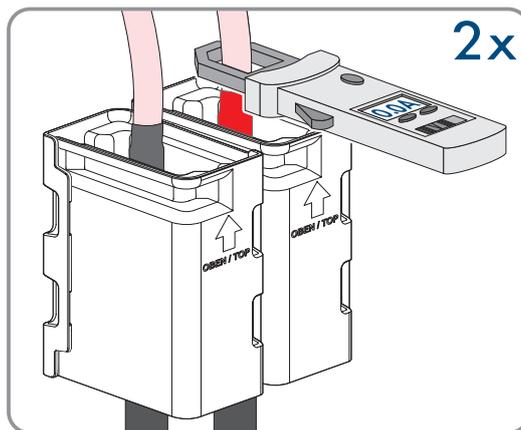
10. Ensure that no voltage is present on the DC voltage measuring points of the pre-charge unit: between **BAT+** and **BAT-**, **BAT+** and **DST-** as well as **BAT-** and **DST-**.
