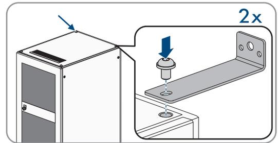
9. Tighten all fastening screws on the cabinet cover (TX55, torque: 20 Nm to 35 Nm).
