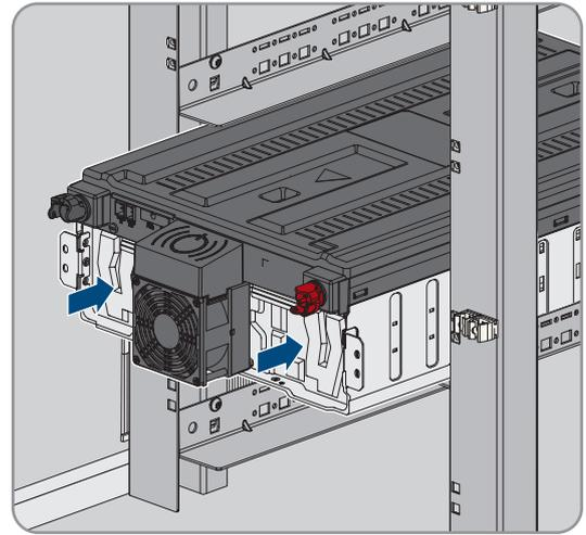
7. Insert the first battery module in the two sliding rails of the lowermost mounting level. Slide in the battery module carefully so the preassembled cage nuts do not become dislodged.
