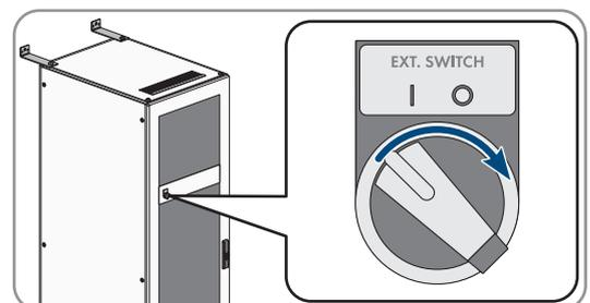
3. Press the **SWITCH** control element on the battery management system.
