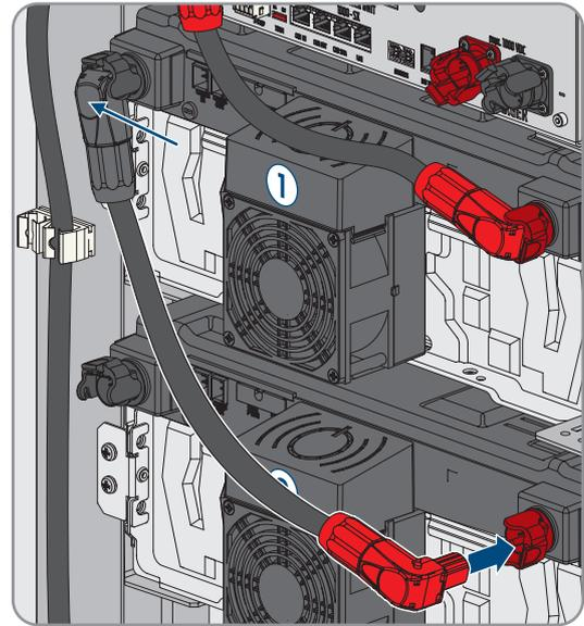
8. Incorporate the rest of the battery modules into the DC cabling within the battery cabinet, working from top to bottom.
