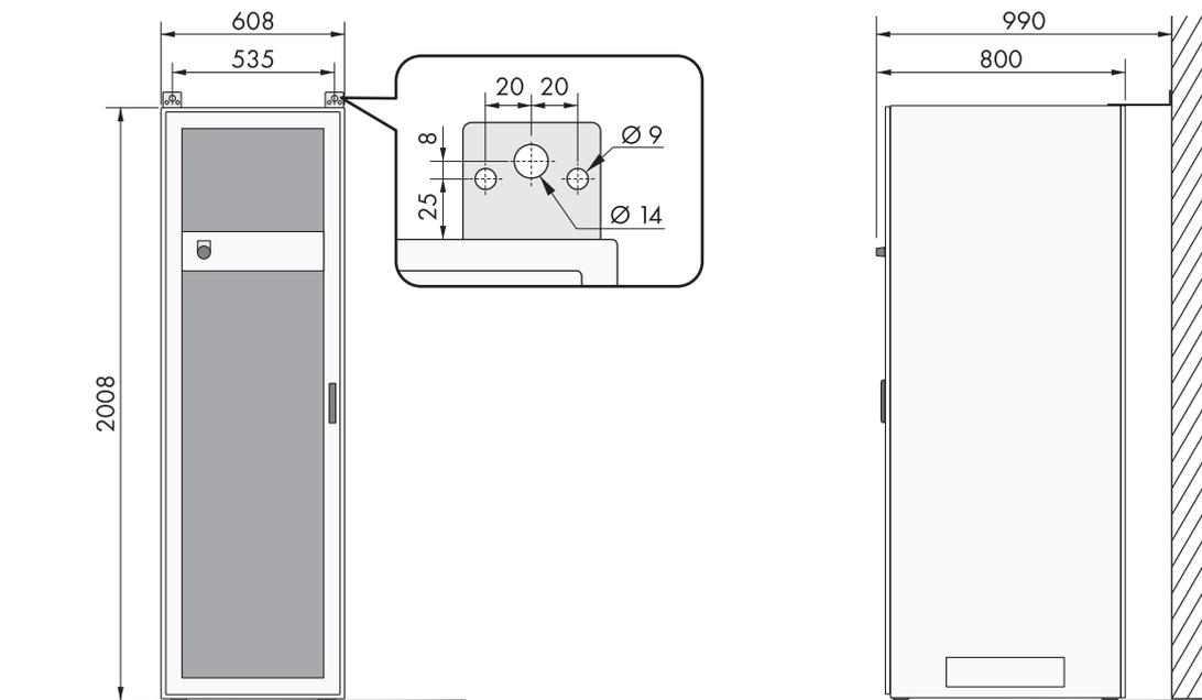
Figure 19: Storage-50-20: Battery cabinet mounting dimensions
