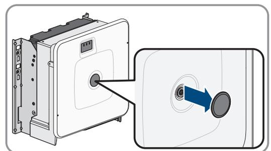
7. Unscrew the screw on the enclosure lid (hex socket, AF10) and remove the enclosure lid.
