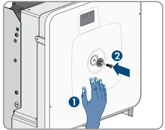
11. Place the cover on the screw in the cover of the enclosure (see Section 15.3, page 174).
