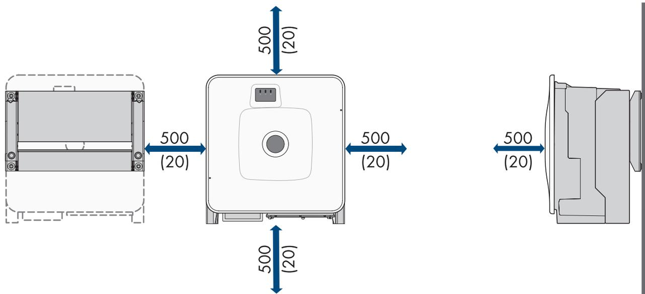
Figure 17: Recommended clearances (dimensions in mm (in))
