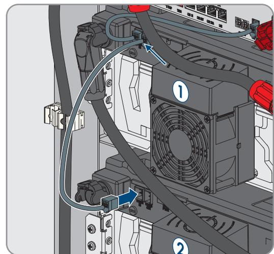
5. Incorporate the rest of the battery modules into the communication cabling within the battery cabinet, working from top to bottom.
