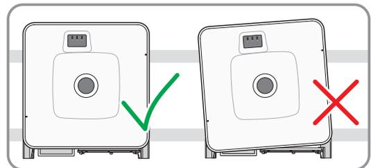
3. Hold the enclosure lid pressed against the enclosure and screw it tight. (Hex socket, AF 10, torque: 18 Nm).
