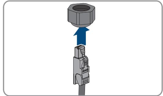
5. Remove the two-hole cable support sleeve from the cable gland.
