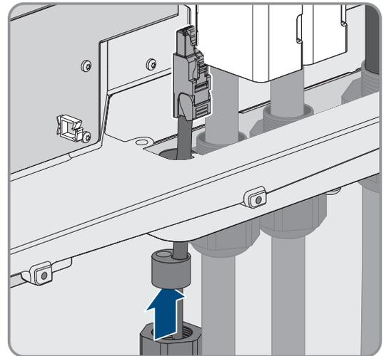
9. When using self-assembly cables, assemble the RJ45 connectors and connect them to the cable (refer to the documentation of the connector).
