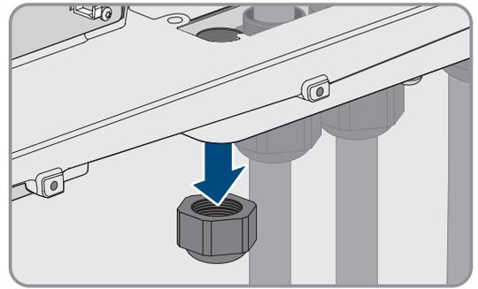
3. Thread a swivel nut over each network cable.
