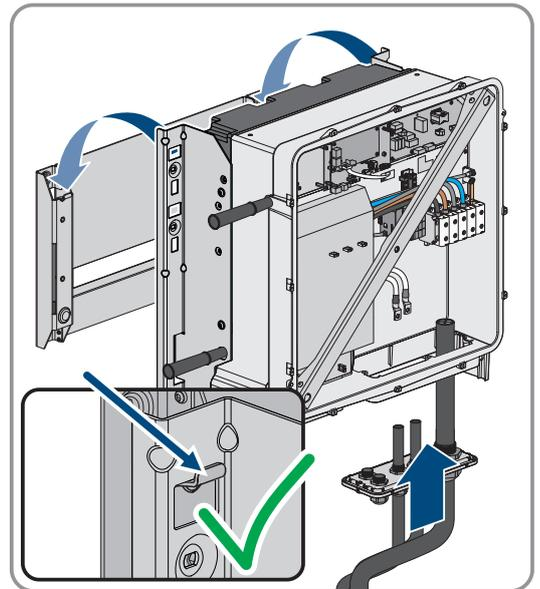
8. Secure the product with 2 screws each on the right and left on the wall mounting bracket (M8x25, TX40, 12 Nm  $\pm$  2 Nm).
