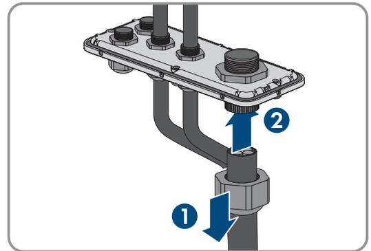
7. Attach the cable glands to the connecting plate.
