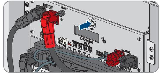
4. Disconnect the DC cables at the **CHARGER+** and **CHARGER-** connections on the battery management system.
