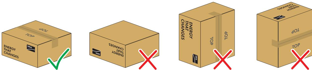
Figure 39: Permitted and prohibited storage positions of a packed battery module
