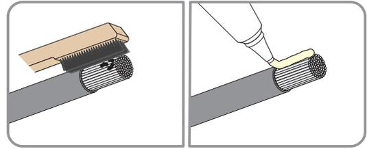
7. Connect PE, N, L1, L2 and L3 to the terminals according to the label. To do so, position each conductor as far as they will go into the corresponding terminal and tighten the screw of the terminal (hex socket AF 5, torque for a conductor cross-section of 16 mm<sup>2</sup> to 95 mm<sup>2</sup>: 20 Nm).
