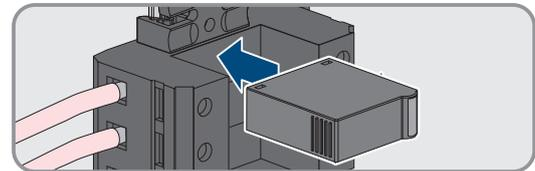
6. Lock the surge arresters by using a screwdriver to turn the latch to the closed position.
