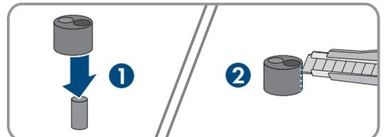
6. Insert each network cable into a 2-hole cable support sleeve.
