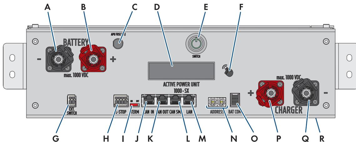
Figure 29: Connections on the battery management system
