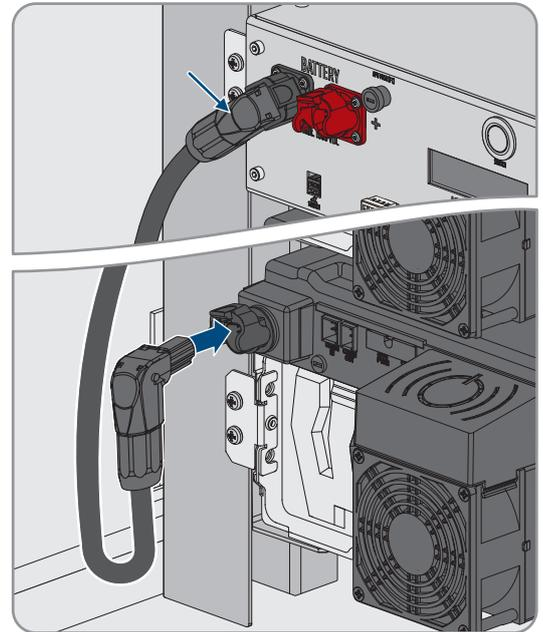
3. Secure the black DC cable on the left-hand side of the battery cabinet. Use the preassembled cable clamps for this.
