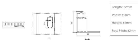
\*This tolerance range applies only to the four-angle distance of the module as indicated above.
