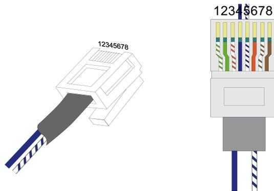
**Step 2** Insert the RJ45 connector to the RJ45 jack.
