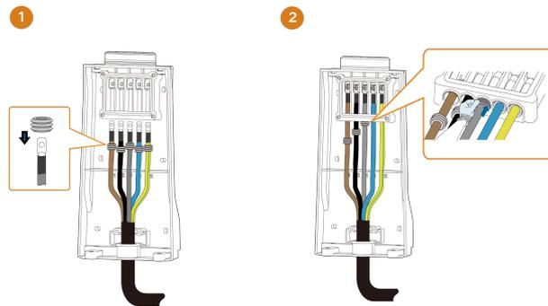
**Step 7** Connect each crimped terminal (OT5.5-4) and tighten them using a M4 screwdriver. (Torque: 1.2 N·m)
