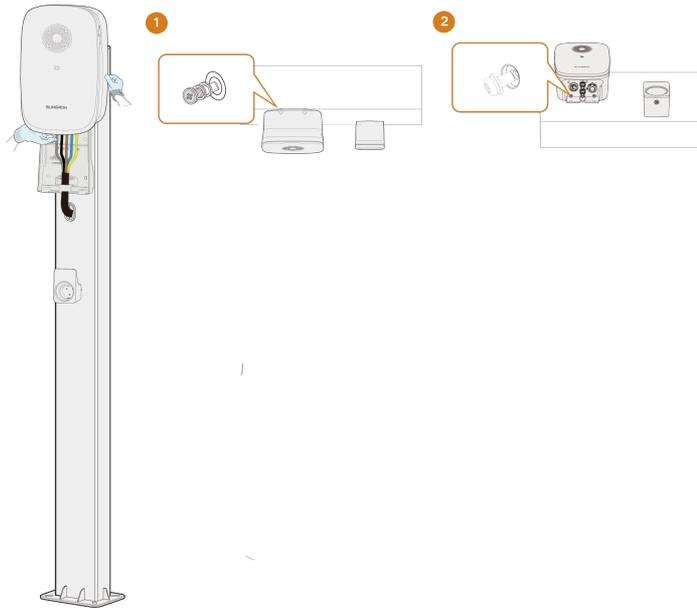
**Step 6** SIM card installation. For details, you can see ["2.5 Wall-Mounting"](#) step4
