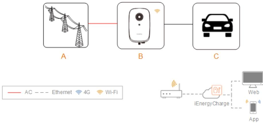
figure 1-3 System topology diagram of EV charger
