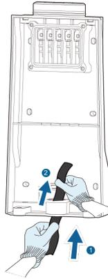
**Step 5** Adjust the cable to a suitable length, and strip off the insulation of the cable to prepare for cable connection terminals.
