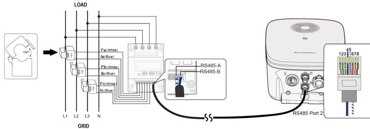
**figure 2-3** Connect to a Smart Energy Meter
