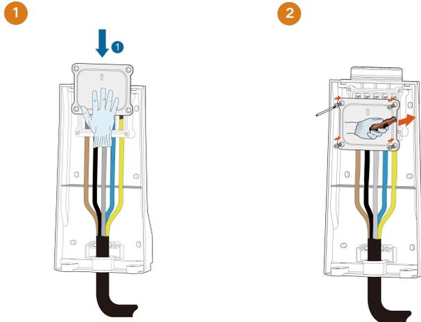
**Step 9** Put the cable fastener in place and tighten the screws to secure it. (M4 screws, torque: 1.2 N·m)
