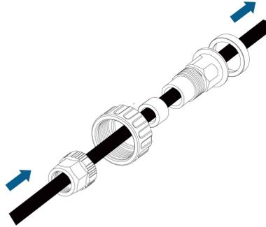
figure 2-2 RJ45 components
