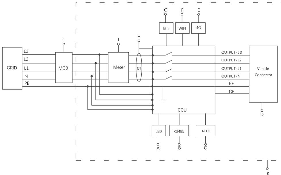
figure 2-1 Circuit diagram
