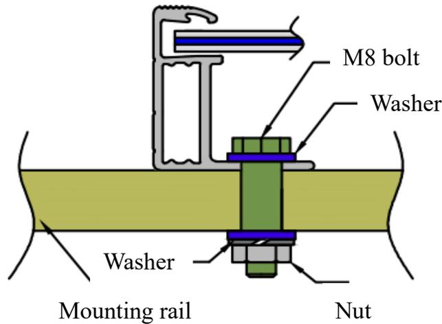
**Fig. 2 Mounting with bolts**
