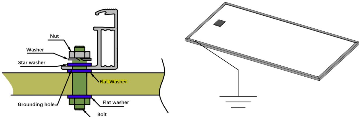
**Fig. 11 Ground connection of PV modules**
