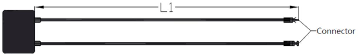
**Fig. 12 (1) The full-cell module junction box**
