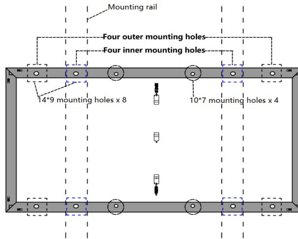
**Fig. 3 Installation with bolt (Four inner mounting holes)**
