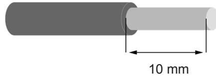
Stripping length of terminals on power stage set (L1, L2, etc.)
