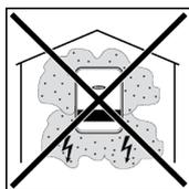
In principle, the Ohmpilot is designed to be dust-tight. However, in areas with high dust accumulation, the cooling surfaces may collect dust and this may impair the thermal performance. In such cases, regular cleaning is required. Consequently, we do not recommend installing the Ohmpilot in places and environments with strong dust formation.
