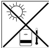
In order to keep warming of the Ohmpilot to a minimum, do not expose it to direct sunlight. Install the Ohmpilot in a protected position. The Ohmpilot must only be installed and operated at an ambient temperature of 0-40°C.
