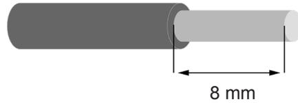
Stripping length of terminals on control board (D+, D-, - and PT1000)
