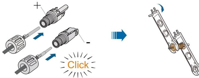
**step 4** Check for polarity correctness.
