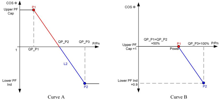
figure 7-18 Reactive Power Regulation Curve in Q(P) Mode
