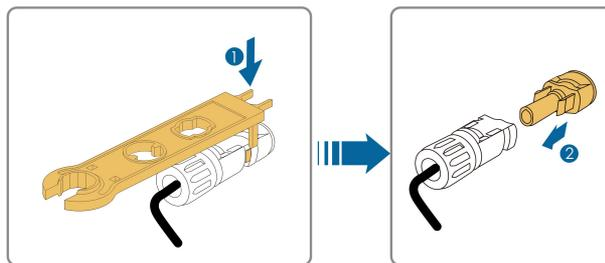
**step 6** Lay the tool in the location of snap and press the tool down to remove the AC connector. Ensure that the AC wiring terminals are voltage-free via a multimeter, and remove the AC wires and communication wires.
