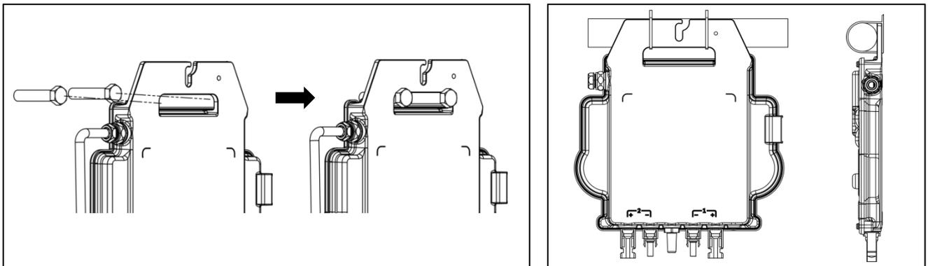
Install the microinverters in proper position to avoid direct exposure to rain, UV or other harmful weather events.
