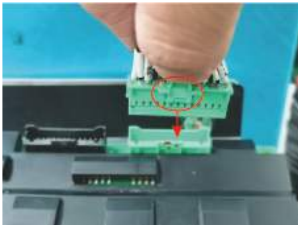
Figure 5-37 Insert the Plug Vertically with the Latch Facing Outward
