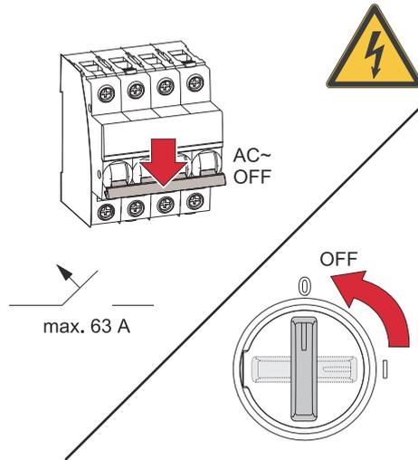
Turn off the automatic circuit breaker. Ensure that the DC disconnecter is in the "Off" switch position.
