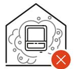
The inverter is designed to be dustproof (IP 66). In areas of high dust accumulation, dust deposits may collect on the cooling surfaces, and thus impair the thermal performance. Regular cleaning is necessary in such situations. We therefore recommend not installing the device in areas and environments with high dust accumulation.
