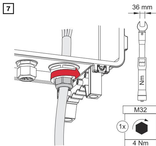
Fasten the union nut of the cable gland with a torque of 6-7 Nm.
