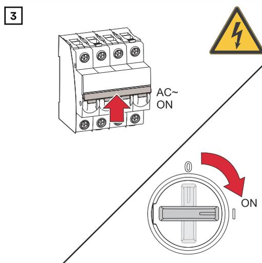
Turn the DC disconnecter to the "On" switch position. Switch on the automatic circuit breaker.
