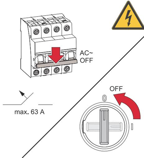
Turn off the automatic circuit breaker. Ensure that the DC disconnect is in the "Off" switch position.
