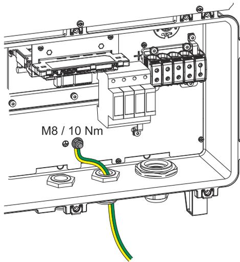
The ground electrode bolt  $\oplus$  allows additional components to be earthed, such as:
