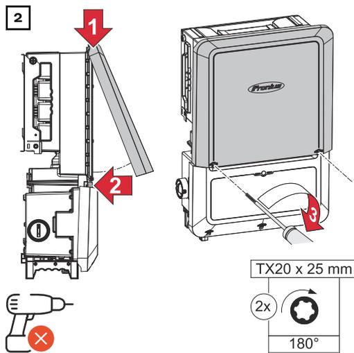
Clip the housing cover onto the inverter from above. Press on the lower part of the housing cover and tighten the two screws by rotating them 180° to the right using a screwdriver (TX20).
