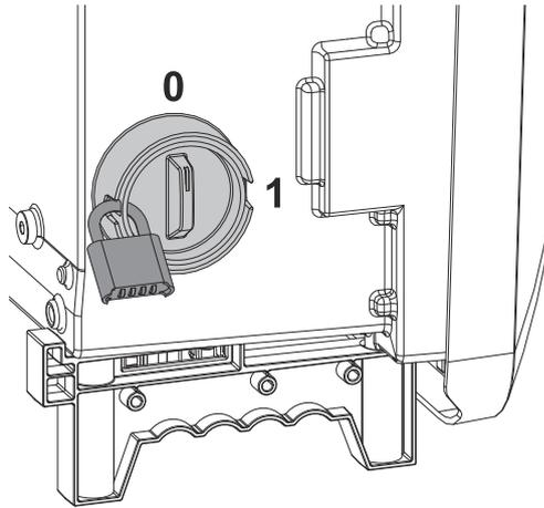
The DC disconnect has 2 switch settings: On / Off.
