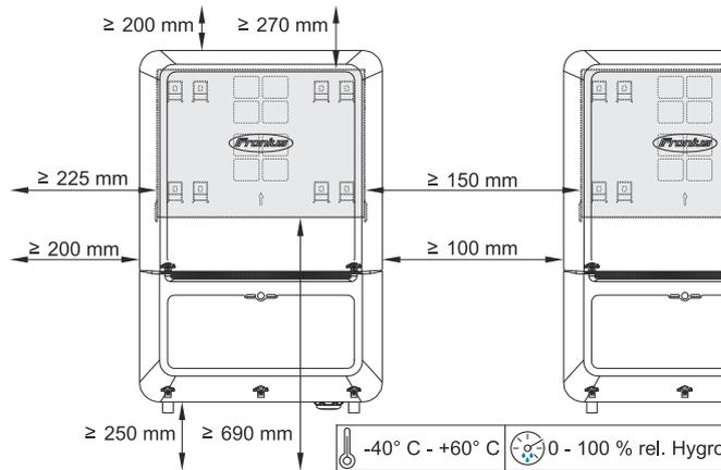
Only install on a solid, non-flammable surface.
