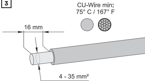
Strip the insulation of the single conductors by 16 mm. Select the cable cross section in accordance with the instructions in [Permissible cables for the electrical connection](#) from page 32.
