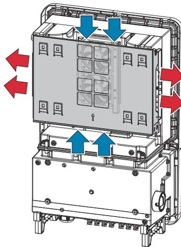
Ambient air is drawn in by the fan on the top and bottom and blown out at the device sides. The even heat dissipation allows several inverters to be installed next to each other.
