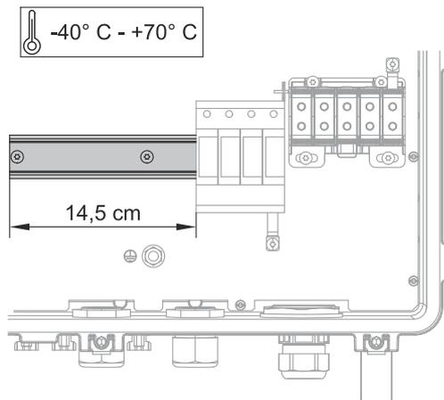
In the connection area there is space for mounting third-party components. Components up to a maximum width of 14.5 cm (8 DU) can be mounted on the DIN rail. The components must have a temperature resistance of -40 °C to +70 °C.
