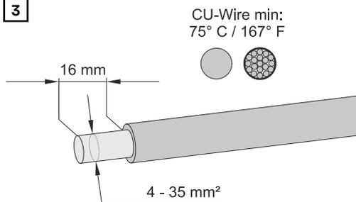
Strip the insulation of the single conductors by 16 mm. Select the cable cross section in accordance with the instructions in [Permissible cables for the electrical connection](#) from page 32.
