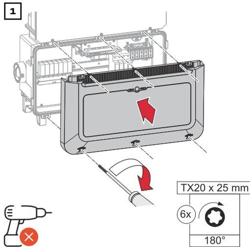
Place the cover on the connection area. Tighten the six screws by rotating them 180° to the right using a screwdriver (TX20).
