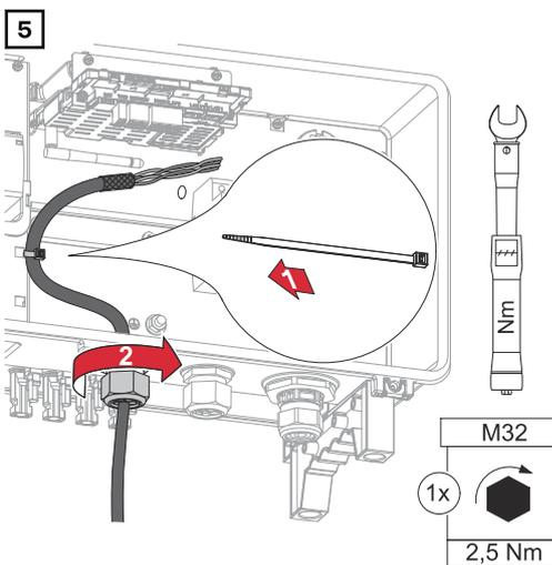
Secure the data cable to the protective cover of the DC SPD surge protective device with a cable tie. Tighten the union nut for the cable gland to a torque of min. 2.5 to max. 4 Nm.
