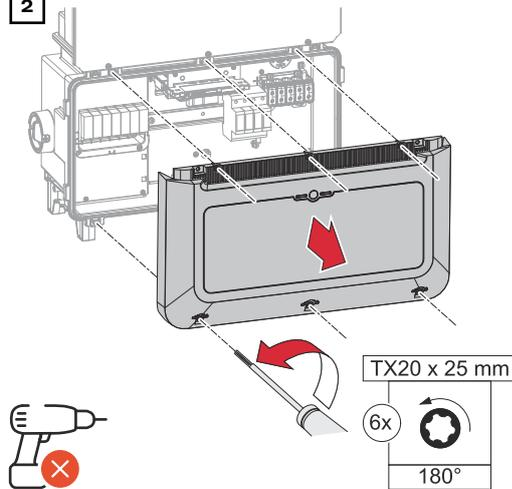
Loosen the six screws of the connection area cover by rotating them 180° to the left using a screwdriver (TX20). Remove the connection area cover from the device.
