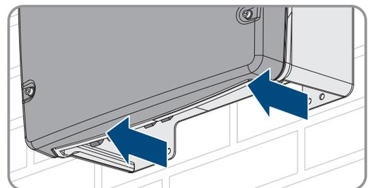
6. Loosen the screws on both sides between the inverter and the wall mounting bracket using an Allen key (AF 5).
