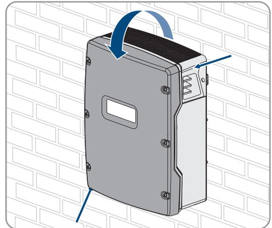
8. Regarding SI6.0H-13 and SI8.0H-13: Remove the inverter by lifting it vertically up and off the wall mounting bracket. For this, use the side recess grips or a steel rod (diameter: maximum 30 mm). Transport the inverter horizontally.
