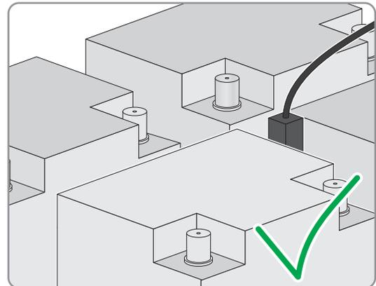
3. Thread both insulated conductors of the sensor through a ferrite included in the scope of delivery and connect to the terminals **BatTmp** on the Sunny Island (see Section 6.6.6 "Connecting BatVtgOut, DigIn, BatTMP and BatCur", page 61). In this case, the polarity is arbitrary.
