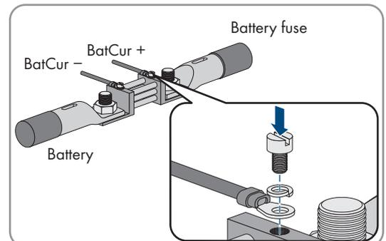
3. Connect the **BatCur-** insulated measuring conductor to the side for connecting the battery on the battery current sensor.
