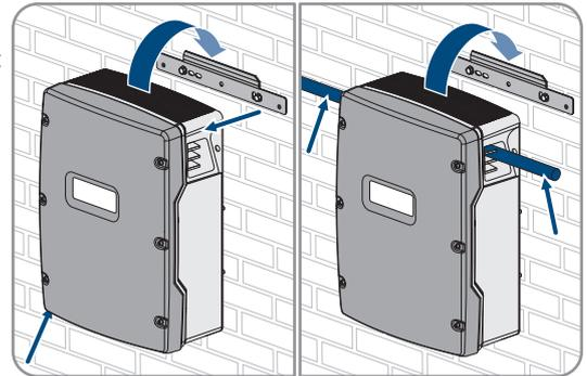
8. Use an Allen key (AF 5) to attach the Sunny Island to the wall mounting bracket on both sides with the M6x10 screws provided (torque: 4 Nm to 5.7 Nm). This will prevent the Sunny Island from being lifted off the bracket.
