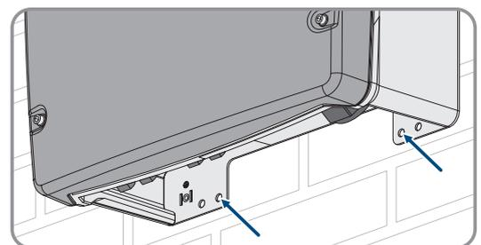
11. Ensure that the Sunny Island is firmly attached.
