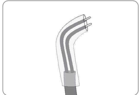
6. Pull the silicone tube over the cable. In this way, the cable is double-insulated.
