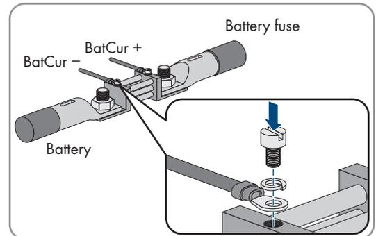
11. Close the battery fuse load-break switch quickly and switch on the inverter.
