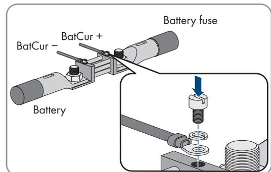
10. Connect the **BatCur-** insulated measuring conductor on the side for connecting the battery.
