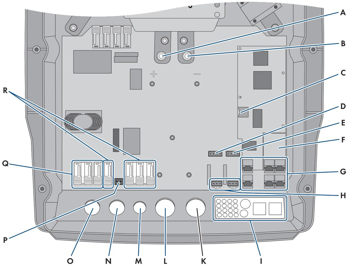
Figure 7: Connection area of the Sunny Island inverter
