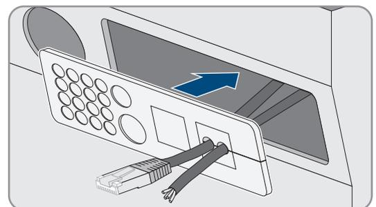
9. Hook the cable feed-through plate into the enclosure opening of the cable feed-through plate and press into the enclosure opening.
