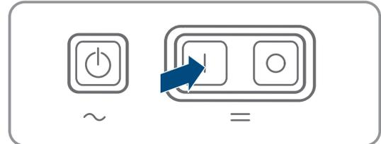
2. For systems with up to three Sunny Island inverters, press and hold the "On" button on the master until an acoustic signal sounds.
