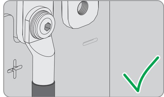
10. Strip off the insulation of the **DC-** cable and mount a terminal lug.
