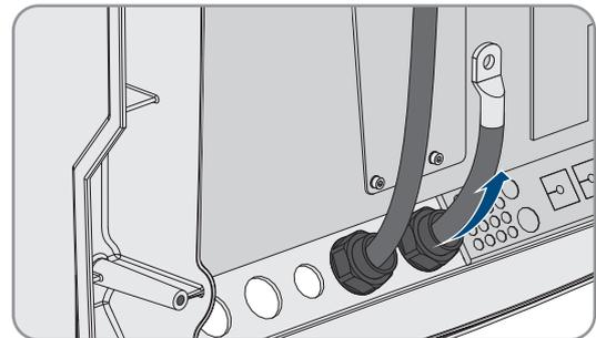
12. Route the **DC-** cable on the side of the protective cover marked with a - symbol.
