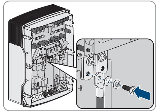
9. Ensure that the entire contact surface of the fender washer is in contact with the terminal lug.
