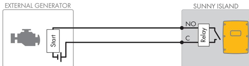
Figure 11: Connecting the Generator Control to Sunny Island
