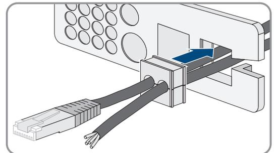
8. Hold the cables and push the cable feed-through plate to the enclosure opening of the cable feed-through plate.
