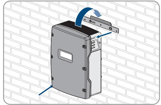
7. Mount the SI6.0H-13 and SI8.0H-13 to the wall mounting bracket. For this, use the side recess grips or a steel rod (diameter: maximum 30 mm). Keep the Sunny Island in a horizontal position when moving it.
