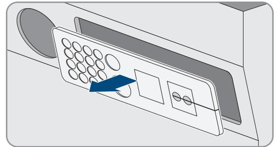
2. Retain the cable feed-through plate for later use.
