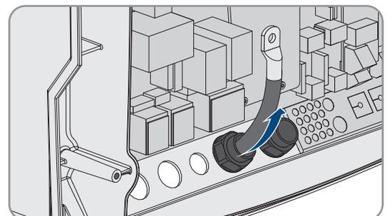
7. Route the **DC+** cable on the side of the protective cover marked with a + symbol.
