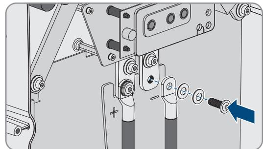
14. Ensure that the entire contact surface of the fender washer is in contact with the terminal lug.
