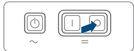
2. For systems with up to three Sunny Island inverters, press the "Off" button on the master.
