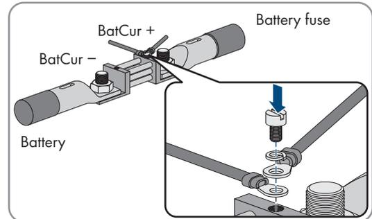
3. Close the battery fuse load-break switch quickly and switch on the Sunny Island.
