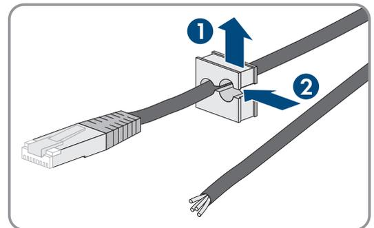
7. Open the cable feed-through plate and insert the cable support sleeves into the cable feed-through plate. Position the flat sides of each cable support sleeve on the flat side in the cable feed-through plate.
