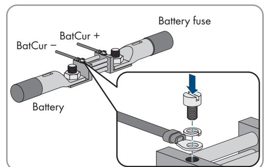
4. Thread both insulated conductors through a ferrite included in the scope of delivery and connect to the terminals **BatCur+** and **BatCur-** on the Sunny Island (see Section 6.6.6 "Connecting BatVtgOut, DigIn, BatTMP and BatCur", page 61).
