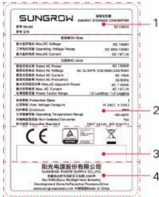
figure 5-1 Nameplate of PCS (SC100CX)
