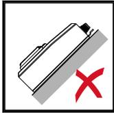
Do not install the Wattpilot on a sloping surface.
