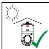
The Wattpilot is suitable for outdoor operation without direct sunlight.
