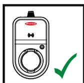
The Wattpilot is designed to be installed vertically on a vertical, level wall.
