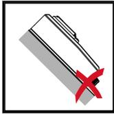
Do not install the Wattpilot on a sloping surface with the connection facing down.
