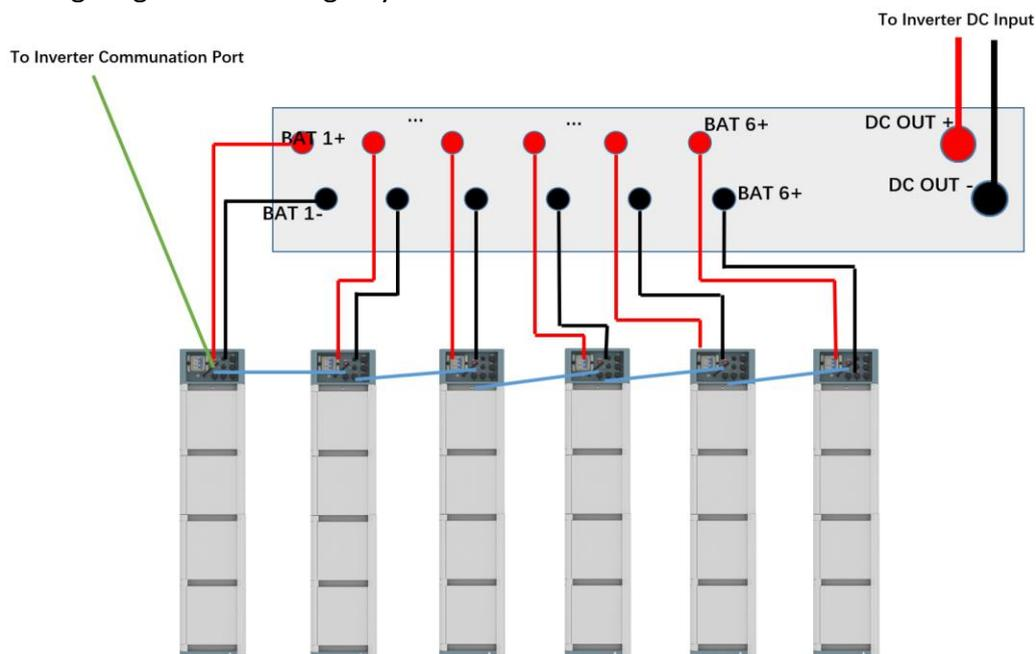
\*It's suggested to use P-Combiner-HV-6 for upto 6 strings, max. 100Amps synchronized continuous operation.
