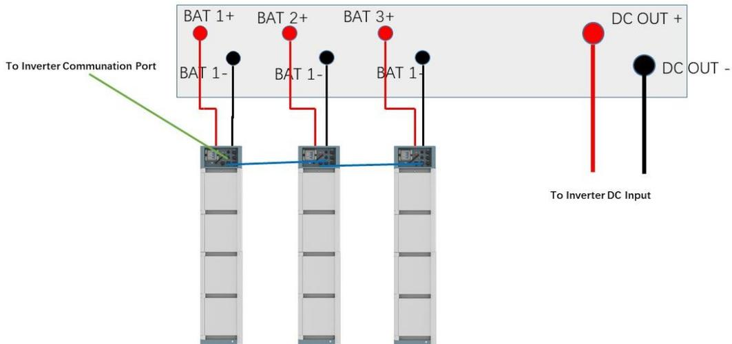
\*It`s suggested to use P-Combiner-HV-3 for upto 3 strings, max. 50Amps synchronized continuous operation.
