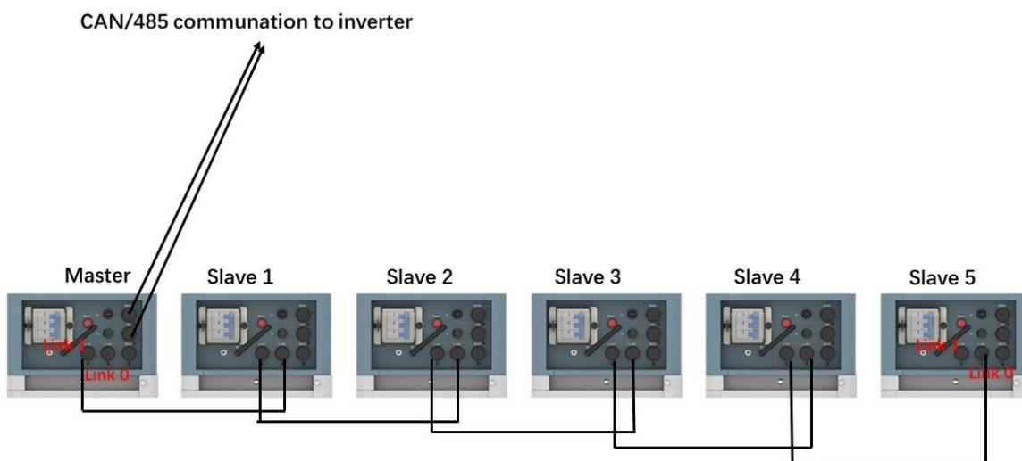
The communication for master/slave string connection shall use a 8pin pin-pin RJ45 cable, connecting from first BMS Link 1 to second BMS Link 0, then from second BMS Link 1 to third BMS link 0(if has), all the way to the last BMS Link 0. The BMS with Link Port 0 EMPTY is defined as the
