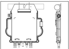
Install the microinverters in proper position to avoid direct exposure to rain, UV or other harmful weather events.
