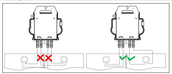
Each PV panel must be carefully connected to the same channel.
