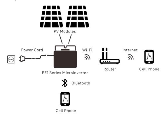
EZ1 series micorinverters have 2 input channels with independent MPPT and high input current and output power to adapt to today's larger power module. Users could directly connect to the Wi-Fi version of EZ1 with their cell phones through Bluetooth and get the real-time data of the solar systems. Besides direct connection, Wi-Fi version of EZ1 could also connect to a router through Wi-Fi and send data to cloud servers for remote monitoring.
