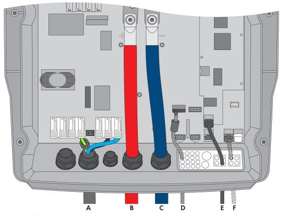
Figure 2: Connection of the Sunny Island
