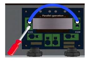
This section applies only, if several Strings with an equal amount of modules are to be connected in parallel and the maximum input current per input therefore exceeds 14A.
