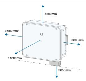
\*When this distance is less than the distance shown, lift the inverter off the stand or wall before maintaining fans.
