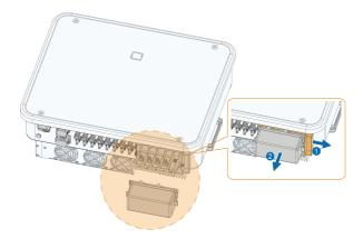
**Step 5** Secure the wires to corresponding terminals. Gently pull the cable backwards to ensure firm connection.
