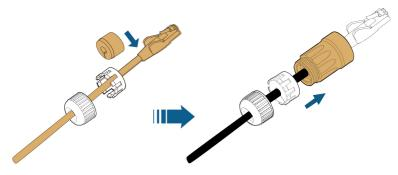
**Step 5** Insert the RJ45 plug into the front plug connector until there is an audible click and tighten the housing. Install the gasket and fasten the swivel nut.
