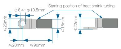
figure 5-3 Specifications of the Crimped OT/DT Terminal
