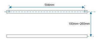
Step 2 Secure the mounting-bracket to the steel u-channel with bolts.
