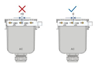
Step 7 Gently pull the cable backwards to ensure firm connection, and fasten the swivel nut clockwise.
