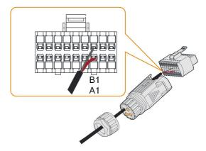
Step 5 Plug the wires into the RS485 terminal according the labels on the bottom of the inverter.
