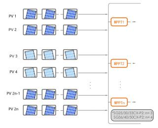
figure 5-4 PV Input Configuratinon
