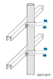
Step 4 Secure the steel u-channels to the pole with bolts and clamps.
