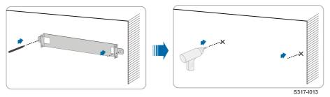
**Step 2** Drill holes with a hammer drill. Clean up the holes, stuff the expansion bolts into the holes, and fix them with a rubber mallet. Use a wrench to tighten the nut to fix the end of the bolt, take off the nut, spring washer and flat washer for spare.
