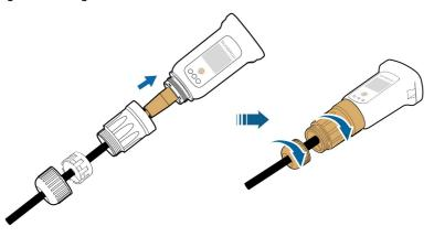
Step 6 Remove the waterproof lid from the COM1 terminal and install WiNet-S.
